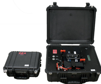
Controller and Drives Boxes
